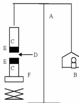
Fig. 1: Bioadhesive force measuring device: (A) modified balance; (B) Weights; (C) glass vial; (D) SA gel; (E) rat tissue; (F) height-adjustable pan.
